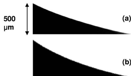
Fig. 6 Two-dimensional meniscus images at an evaporation rate of 9.35 \times 10^{-7} kg/s and a heat flux of 820 W/m 2 in different channel widths: (a) 500 \mu\text{m} and (b) 600 \mu\text{m}
